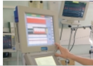
The PulseCO displays real-time beat to beat critical parameters, which are plotted on the monitor
